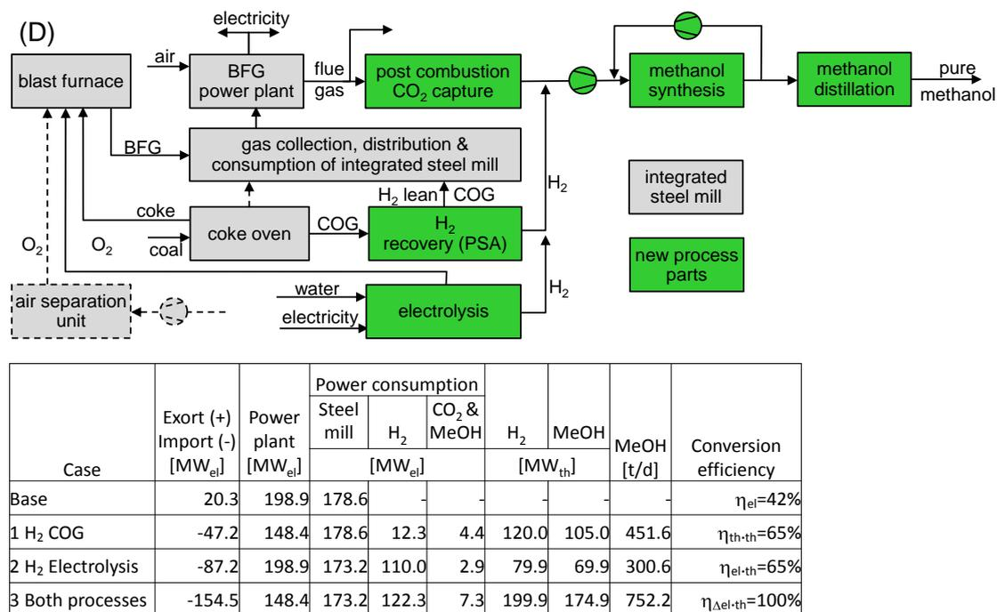
**Figure 7: Energy Balance of Steel-Methanol Plant Design with Post Combustion Capture, Electrolyzer, and CO<sub>2</sub> Methanol Synthesis**
