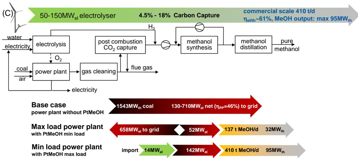
**Figure 5: Energy balance of Power Methanol Plant Design with Post Combustion Capture, Electrolyser, and CO<sub>2</sub> Methanol Production.**
