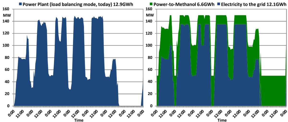
**Figure 6: Actual Operational Load of a Coal Power Plant of 150 MW<sub>el</sub> Plant in Germany (Left ) and Possible Increase of Operational Load by Power to Methanol for Efficient Operation (Right)**
